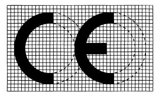
If the marking is reduced or enlarged, the proportions given in the above graduated drawing must be respected.
